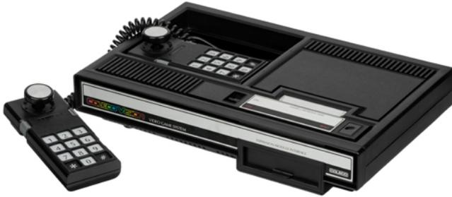
Developed by Coleco Industries, Inc., the Colecovision was manufactured in the United States, specifically in West Hartford, Connecticut. Its construction process involved utilizing a Z80 microprocessor, a state-of-the-art hardware component at the time, which allowed for its superior graphics and sound capabilities.
